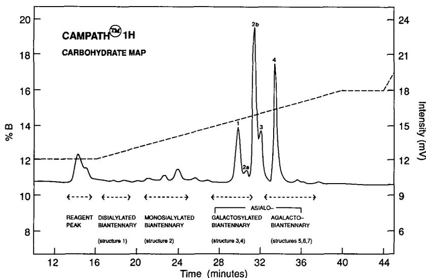
Fig. 1. Reversed-phase HPLC map of oligosaccharides released from CAMPATH-1H. Conditions: column, Spherisorb S3-ODS 2 (15 cm  $\times$  4.6 mm; Phase Sep); mobile phase A, 0.1 M sodium phosphate (pH 7); mobile phase B, acetonitrile; mobile phase gradient as indicated; flow rate, 0.7 ml min<sup>-1</sup>; wavelength, 245 nm; room temperature.
