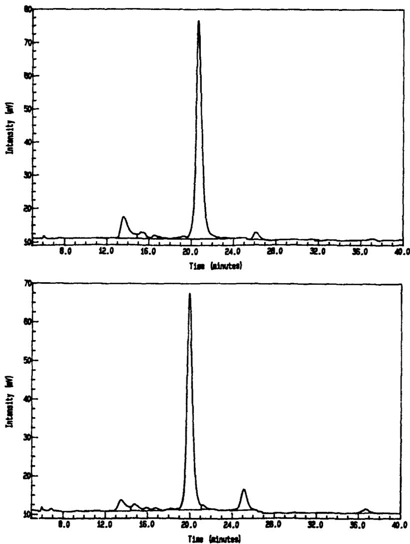
Fig. 4. (a) Carbohydrate map of GPF-released sugars from human transferrin (0.125 mg); (b) carbohydrate map of purchased library of released sugars (by hydrazinolysis) from human transferrin (5 mg).
